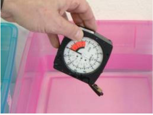
A hand is holding a black altimeter with a white dial and a red needle. The altimeter is positioned over a pink plastic container. The dial has markings for feet and meters, and the needle is pointing to approximately 1000 feet.     | <p>STEP 4</p> <p>When soak time is completed, dunk the soaked altimeters at least five times in the same container.</p> <p>Shake off excess water by hand.</p> |
