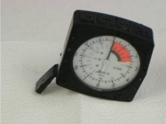
A black altimeter with a white dial and a red needle is shown resting on a white surface. The battery door on the left side is open. The dial has markings for feet and meters, and the needle is pointing to approximately 1000 feet. | <p>STEP 6</p> <p>Place rinsed altimeters right side up with battery door open, on a stable surface to drip dry.</p>                                            |
