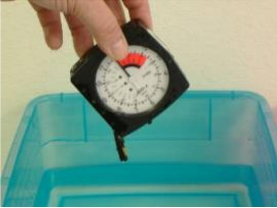
A hand is holding a black altimeter with a white dial and a red needle. The altimeter is positioned over a blue plastic container. The dial has markings for feet and meters, and the needle is pointing to approximately 1000 feet.    | <p>STEP 5</p> <p>Place the drained altimeters into the second container and again dunk at least five times.</p>                                                |
