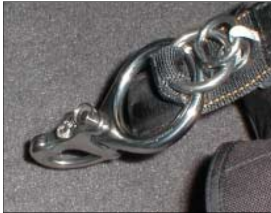
Optional Main attachment fitting: Stainless Steel Snap Shackle (Wichard p/n 2272) with a Butler custom, machined Stainless (17-4) ring. This hardware has an approximate safe working load of 7,000 lb.
