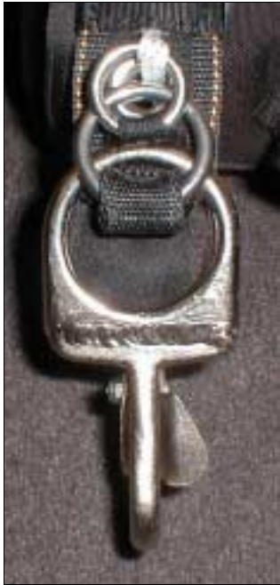
Standard harness attachment configuration consisting of a welded RW-10 / MS22042 Butterfly Snap (either cadmium or nickel plated). This hardware has an approximate safe working load of 3,500 lb.
