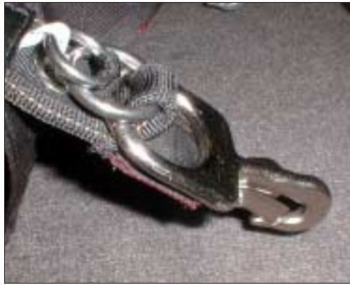
Standard harness attachment configuration consisting of a welded RW-10 / MS22042 Butterfly Snap (either cadmium or nickel plated). This hardware has an approximate safe working load of 3,500 lb.
