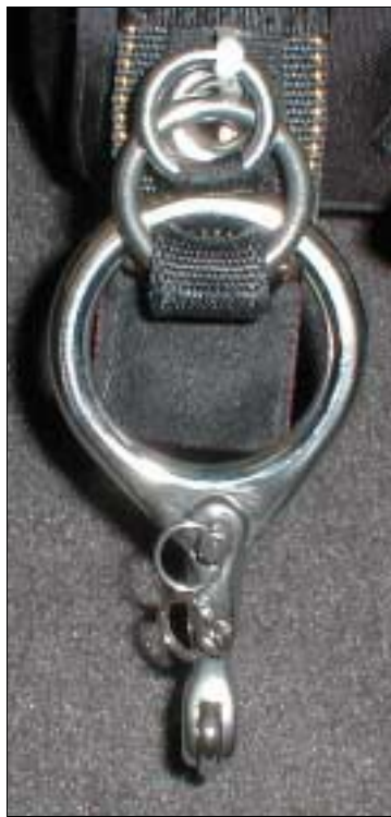
Optional Main attachment fitting: Stainless Steel Snap Shackle (Wichard p/n 2272) with a Butler custom, machined Stainless (17-4) ring. This hardware has an approximate safe working load of 7,000 lb.
